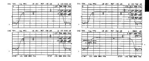
Figure 2-6. Example of Coupled and Uncoupled Markers
