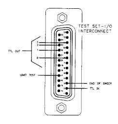
Figure 5-3. Pin Locations on IO Interconnect
