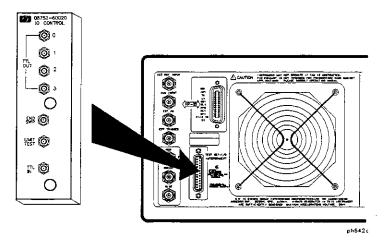
Figure 5-4. IO Control Adapter
