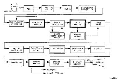
Figure 3-5. Data Processing Flow Diagram
