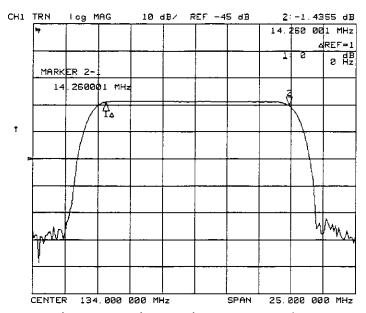
Figure 2-5. Marker 1 as the Reference Marker
