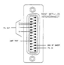
Figure 1-4. Test Set Interconnect Pin-Out
