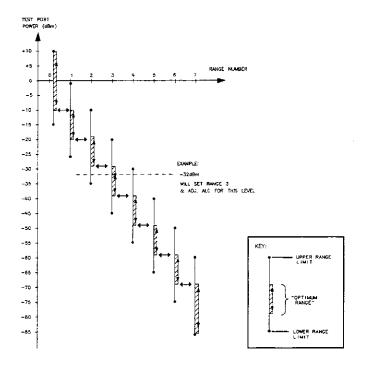
Figure 5-2. Power Range Transitions in the Automatic Mode
