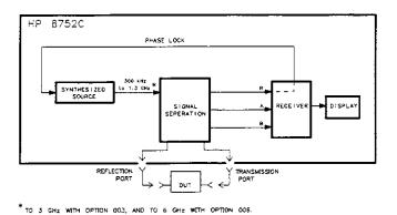
Figure 5-1. Simplified Block Diagram of the Network Analyzer System
