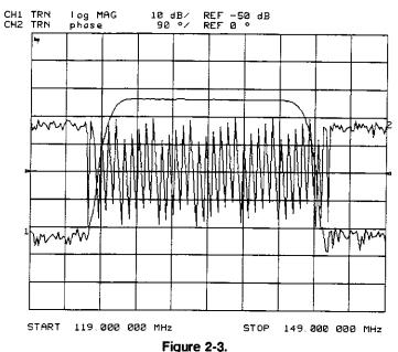
Example of Viewing Both Channels with a Single Graticule
